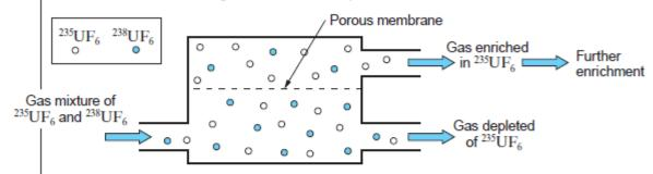
During this stage, the mixture is enriched by a factor that can be calculated using:
